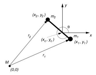
Consider two test masses,  $m_1$ ,  $m_2$  connected by a massless rigid rod of length d, in orbit about a mass,  $M >> m_1, m_2$  as shown in the figure above. Let  $(x_i, y_i), i = 1, 2$  be the coordinates of the two test masses, let  $(x_c, y_c)$  be the coordinates of the dumbbell's center of mass, and let  $\theta$  be the angle the rod makes with the x-axis. Defining
